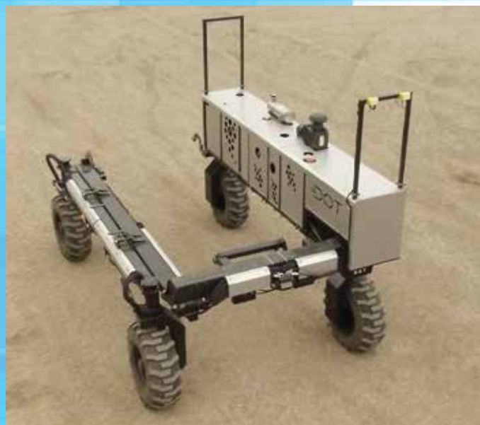
The DOT Power Platform is designed to work with multiple types of farming implements, such as seeders, grain carts and sprayers. Photo courtesy of DOT Technology Corporation.
