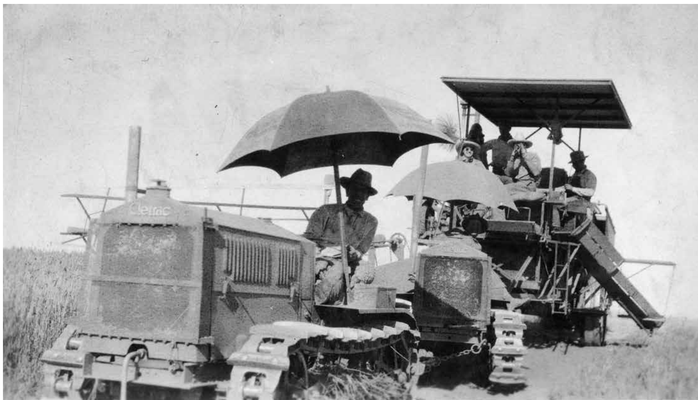
Tractor and combine near Colfax, Wash., circa 1930. Adolf Harder drove one of the tractors; the other men are unidentified. Two tractors were needed to pull one combine. They had to turn in unison because if they didn't, the tracks would come off the tractor causing a delay of several hours. The tractor is a Cletrac 20. Creator is unknown. Photo courtesy of the Whitman County Library. (WCLCF222, washingtonruralheritage.org)
