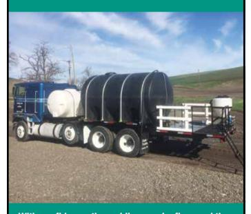
With confidence, the welding sparks flew, and they made it work! With a 3000 gal. tank, 710 Fert. tank and 8 ft. mixing platform with foldable ladder, it's already making their jobs easier. Thanks JB and Lane Heaten on the great fab. work.
