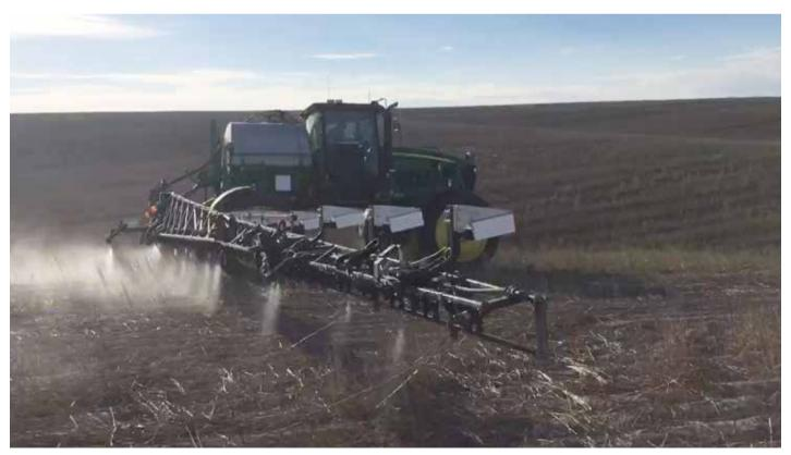
The WEEDit equipment uses chlorophyll-sensing technology to identify weeds and apply herbicides only where needed as demonstrated in this photo courtesy of Jason Emerson of the Odessa Trading Company/Vantage-PNW.
