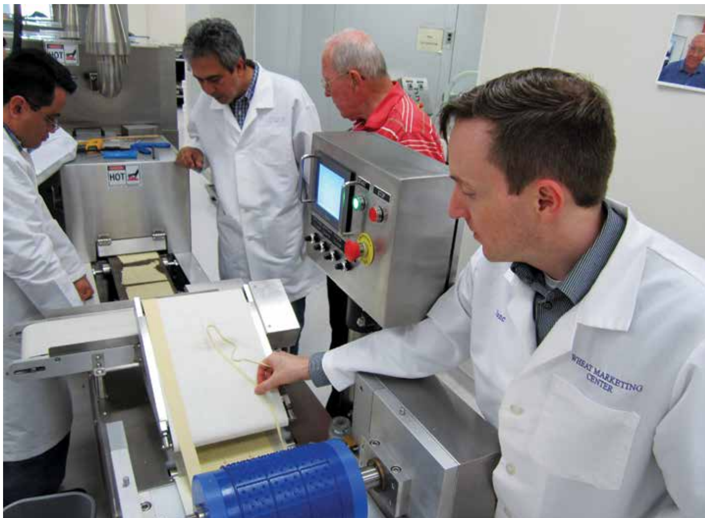
During a visit to the Wheat Marketing Center, Mexico City-based Marcelo Mitre works on the pilot-scale cracker line that allows companies to test formulations without having to shut down an entire line at one of their plants.
