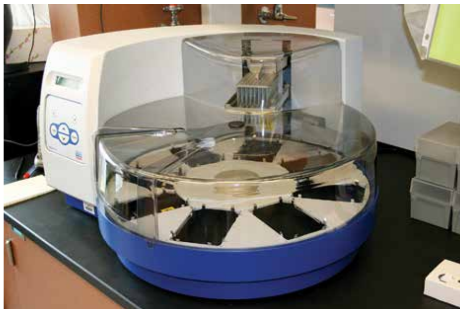
(Above) The Biosprint 96 is a DNA extraction machine that allows Washington State University researchers to extract DNA from 96 different leaf samples simultaneously, which can then be used for molecular analysis. The plots (below) show a wheat line with three genes for rust resistance (on the left) as determined through the use of DNA markers, and a plot of a wheat line without genes for resistance.
