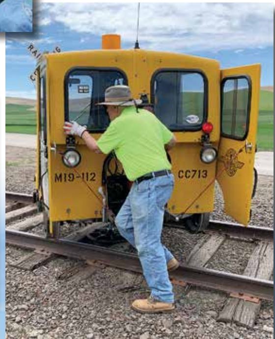
(Above) People couldn't help smiling and waving as the cars rode past. (Below) Many speeder cars have a hydraulic foot that extends down and lifts the car off the tracks so it can easily be turned around.
