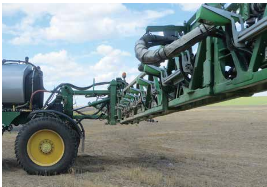
A sensor system from just outside Ritzville, Wash. The sensor heads are the evenly spaced green boxes on the front of the boom.
