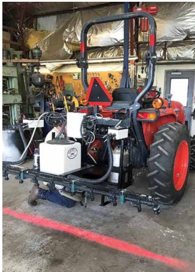
The system Washington State University researchers have been evaluating is an eight-foot boom with two sensors. The sensor heads are the white boxes. The sensor emits near infrared light, which is visible on the concrete floor.
