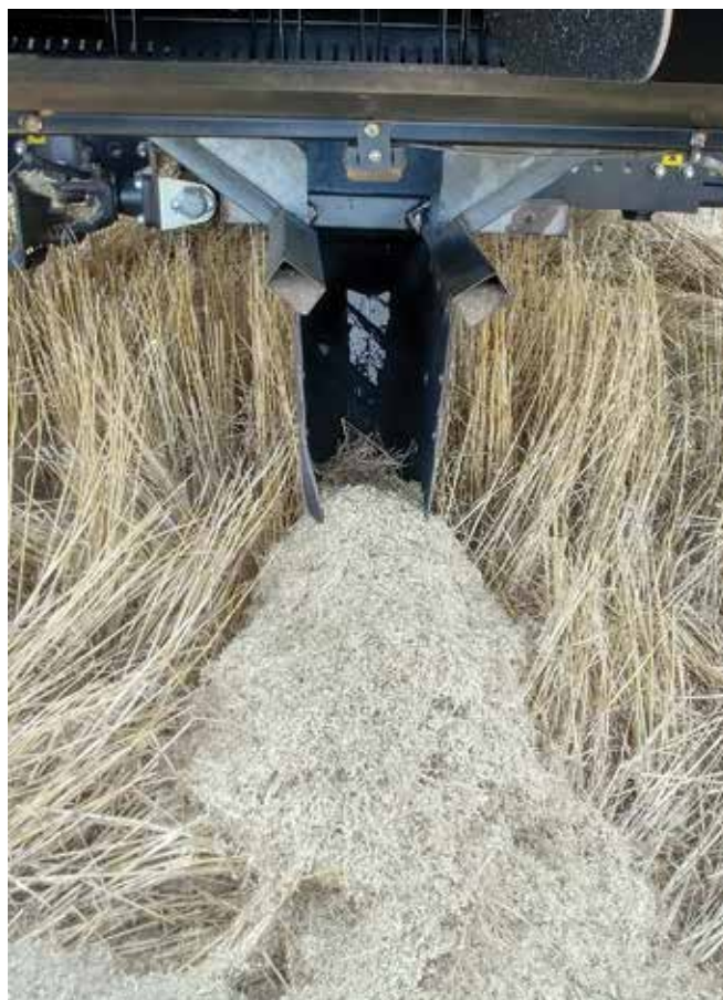
Chaff lining, where the chaff and weed seeds are laid down in a narrow line behind the combine. Weed seeds in the chaff struggle to survive in this inhospitable environment.
