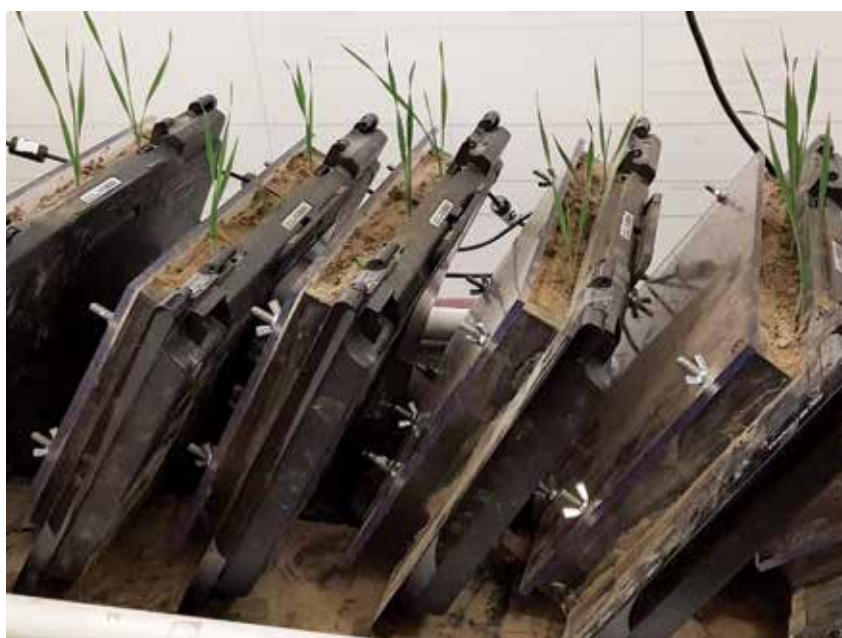
Figure 1. Scanner based rhizoboxes allow for high resolution imaging of plant disease root interactions.
