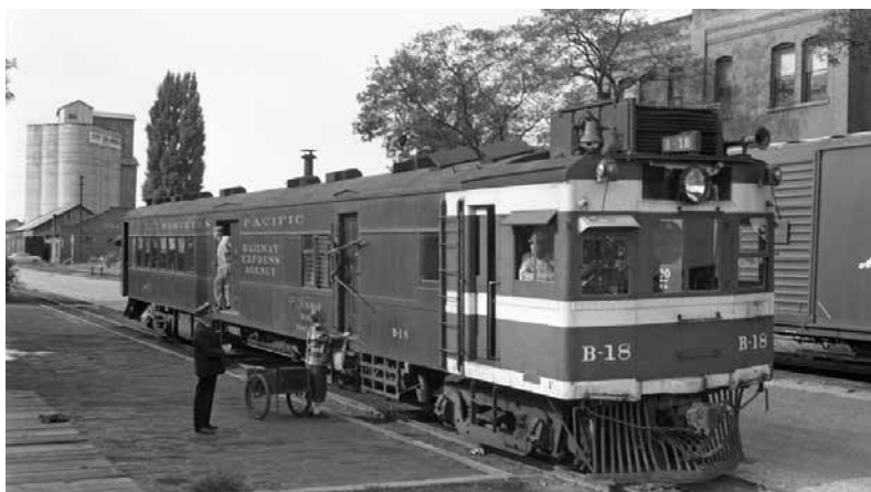
This picture shows the apparatus on the outside of the train that was used to hand mail off to the station. Photo by Wade Stevenson, courtesy of Milwaukee Road Historical Association and the Northern Pacific Railway Historical Association Archives.
