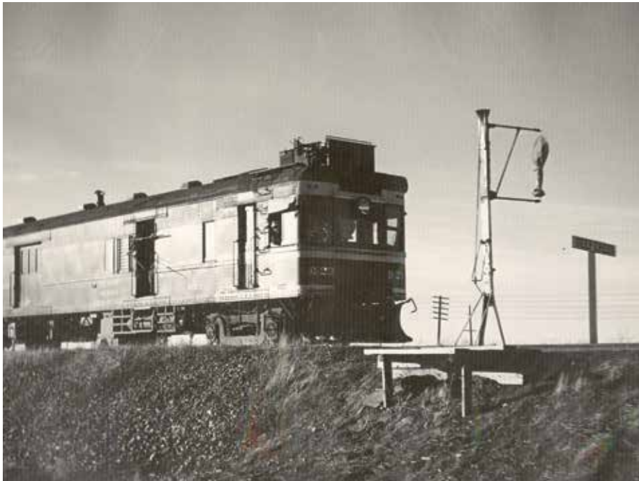
Train #316 at Deep Creek, Wash., showing the train ready to snatch the mail sack from the mail crane circa 1950-51. Photo by Philip Hastings, courtesy of Bruce Butler.
