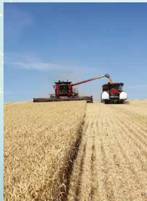
(Above) Unloading the combines on the go into a bank-out wagon saves time because the combines don't have to stop harvesting or drive to where the trucks are waiting, usually near edge of the field. The Zwainzes truck their wheat to the HighLine Grain Growers elevator in Reardan (below).
