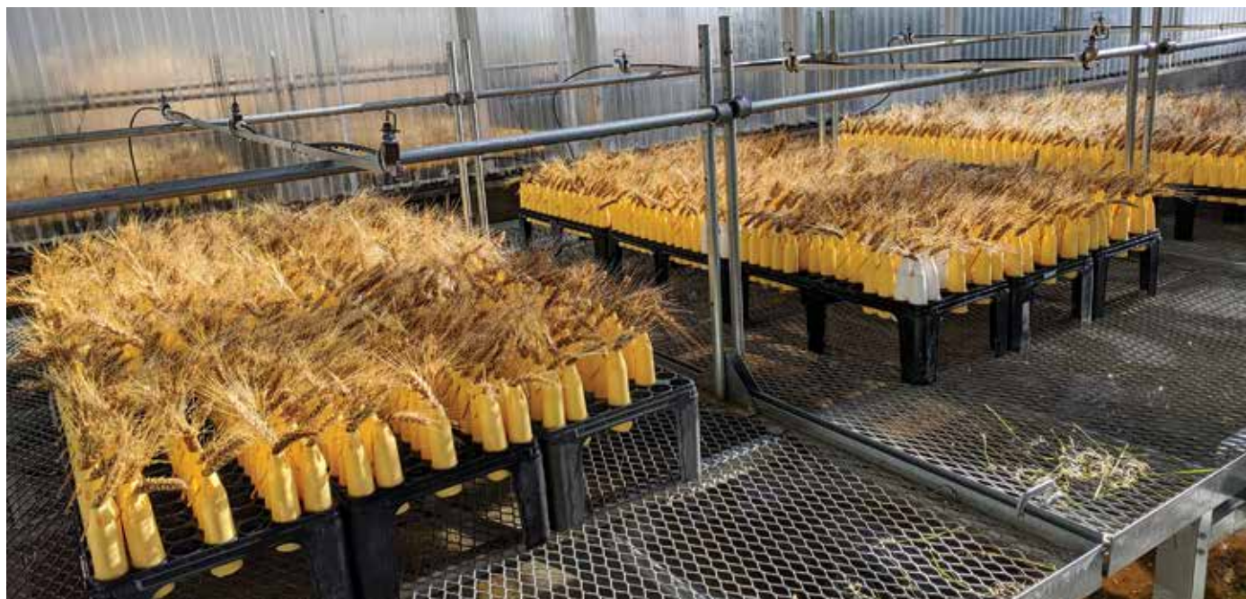
The spike-wetting test is used to assess the preharvest sprouting resistance of wheat varieties.
