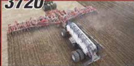
The 3720 Disk Drill has 7.5", 10" or 12" spacings available with 30 ft. to 70 ft. widths.
