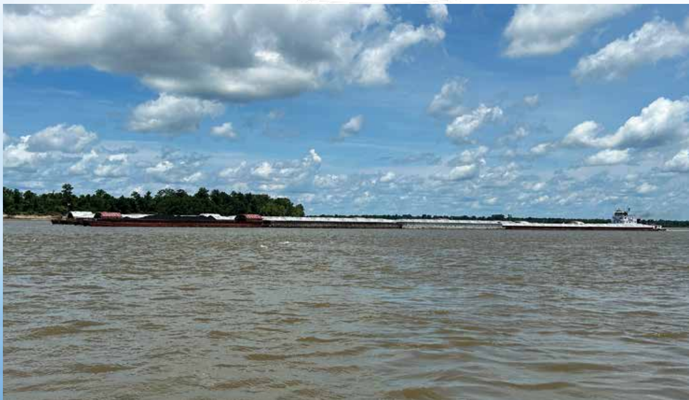
Tows on the Mississippi are big, much bigger than the four-barge tows common on the Columbia and Snake rivers. An average tow on the lower Mississippi River is 30 barges. The river makes a big bend at Vicksburg, Miss., right before passing underneath the Old Vicksburg Bridge. The currents and shifting sandbars mean navigation is tricky through this stretch, and it's not unusual for vessels to end up hitting the bridge.
