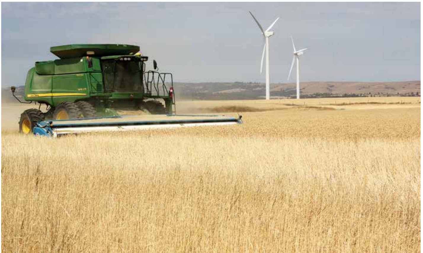
Klickitat County wheat grower Andy Juris uses a stripper header that leaves more plant residue in his fields than regular headers do. A new Natural Resources Conservation Service practice can help growers who want to invest in this type of equipment.
