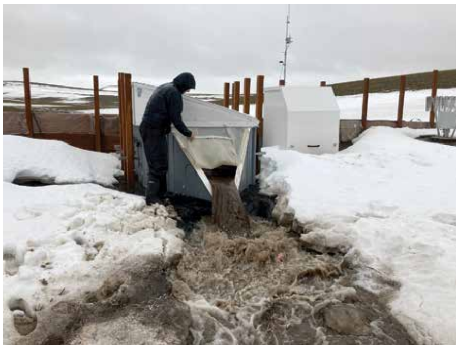
An H-flume recording surface runoff on February 23, 2025, flow at the Cook Agronomy Farm. One liter water samples are collected from the runoff by automated water samplers. These samples are analyzed from sediment, nitrate, dissolved and particulate phosphorus. Photo by Erin Brooks.
