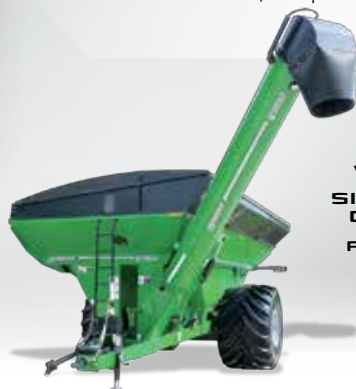
AVALANCHE DUAL-AUGER GRAIN CART FROM 2,500- TO 1,100- BUSHEL CAPACITIES
