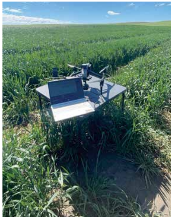
A typical flight setup needed to capture drone images in a winter wheat field.
